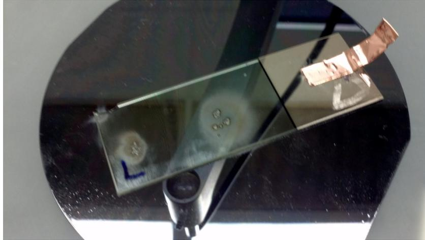
Figure 18. Dielectric breakdown that occurred in PDMS thin film.
