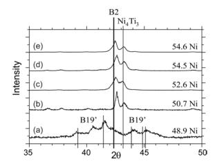
**FIGURE 1.** X-Ray Diffraction of the As-Quenched Ni-Ti Alloys. Vertical lines indicate the peaks corresponding to various phases.
