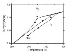
**FIGURE 3.** Fig. 2 expanded to show the martensitic hysteresis.  $M_s$  is 323K,  $A_f$  is 363K and  $M_f$  is below 298K, near the intersection of the cooling and heating curves. Arrows indicate the thermal path.
