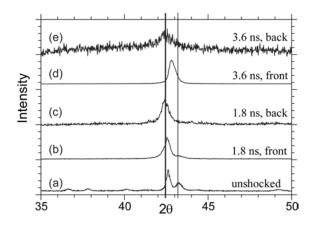
**FIGURE 7.** XRD of AQ (a) and shocked (b-e) 50.7 Ni. The thick vertical line denotes B2; the thin line denotes Ni<sub>4</sub>Ti<sub>3</sub>, which is gone after loading. The shots had initial shock pressures of 15 GPa (b,c) and 7 GPa (d,e). The 2nd shot (d,e) used no window.
