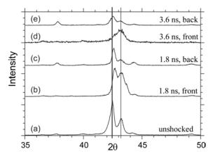
**FIGURE 8.** XRD scans of AQ (a) and shocked (b-e) 54.6 Ni. The thick vertical line denotes B2; the thin line denotes Ni<sub>4</sub>Ti<sub>3</sub>, which increased on the front faces after loading. The shots had initial shock pressures of 19 GPa (b,c) and 21 GPa (d,e), respectively.
