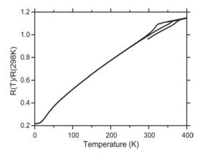
**FIGURE 2.** Resistivity of 48.9 Ni. R(298K)=1.92 x 10<sup>-4</sup> ohm-cm.
