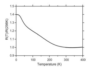
**FIGURE 4.** Resistivity of 50.7 Ni, showing no hysteresis and also a negative temperature dependence.  $R(298K)=1.07 \times 10^{-4}$  ohm-cm.
