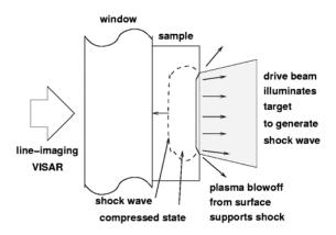
FIGURE 5. Schematic of TRIDENT direct drive experiments.
