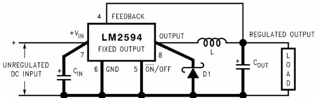
**Figure 5: Voltage Regulator circuitry – shown above, the circuitry required to regulate the voltage from 48V down to 5VDC. The circuit for the 12V regulator is the same, only required different values for the capacitance values on  $C_{IN}$  and  $C_{OUT}$ .**
