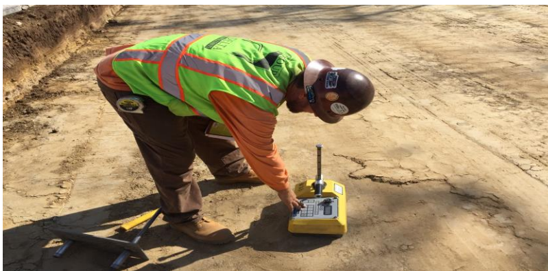
Exhibit B: Nuclear testing for soil compaction
