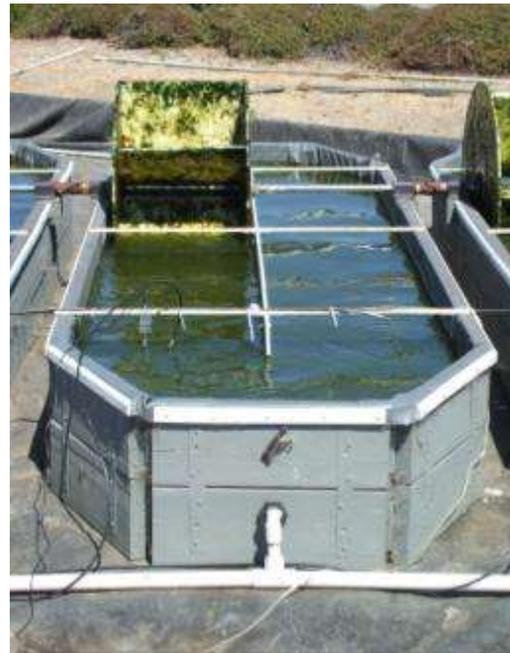
Figure 4. HRAP (unpublished photograph, July 28, 2010). The PVC pipe that collected the effluent is shown at the bottom of the picture, and the in-line paddlewheels are at the top of the picture. The four ponds were constructed next to each other and were labeled Pond 1, 2, 3, and 4 respectively.
