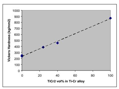
**Figure 2.** Vickers hardness versus the volume percentage of the TiCr<sub>2</sub> intermetallic phase in the alloy. The strength and hardness are a function of the type and amount of phases present.
