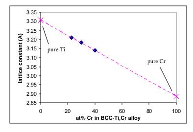
**Figure 3**. The β-BCC lattice constant versus Ti-Cr alloy composition. The dotted line represents Vegard's Rule and is based on the lattice constants for pure Ti and  $Cr^2$ . Extrapolations of the experimental lattice constants to the Ti-Cr alloy composition are quite accurate.
