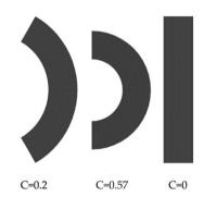
Fig. 2. Two curved fibers and one straight fiber.
