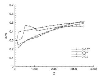
Fig. 3. Lateral migration of curved and straight fibers at the density ratio of 1.05, the Reynolds number of the curved fibers is Re = 31.2, the Reynolds number of the straight fiber is Re = 37.7. The diamond and square symbols represent the curved fibers with their concave sides facing the left wall. The triangle symbol represents the curved fiber with its convex facing the left wall. The X-axis is the position of fiber mass center.
