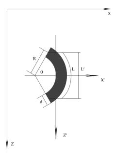
Fig. 1. Curved fiber and its parameters.
