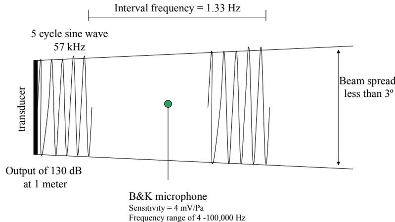
**Figure 4 - Acoustic transducer and microphone details.**
