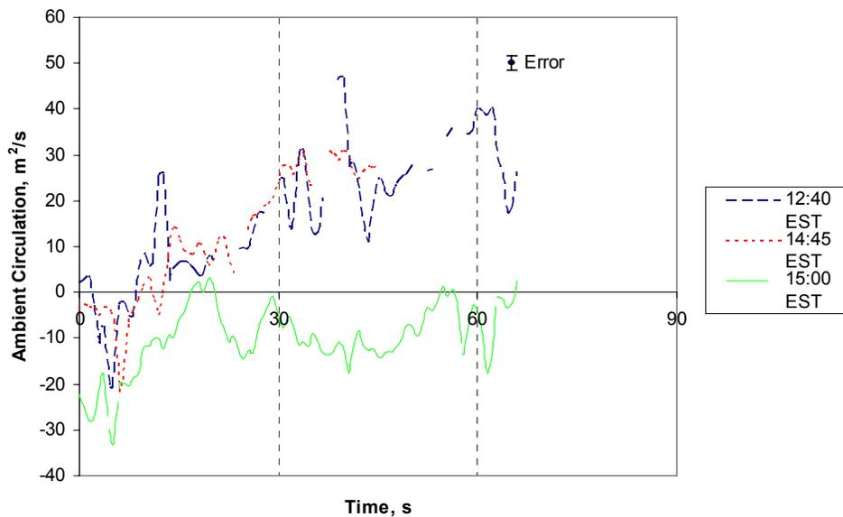
**Figure 8 - Ambient circulation measurements due to cross wind.**
