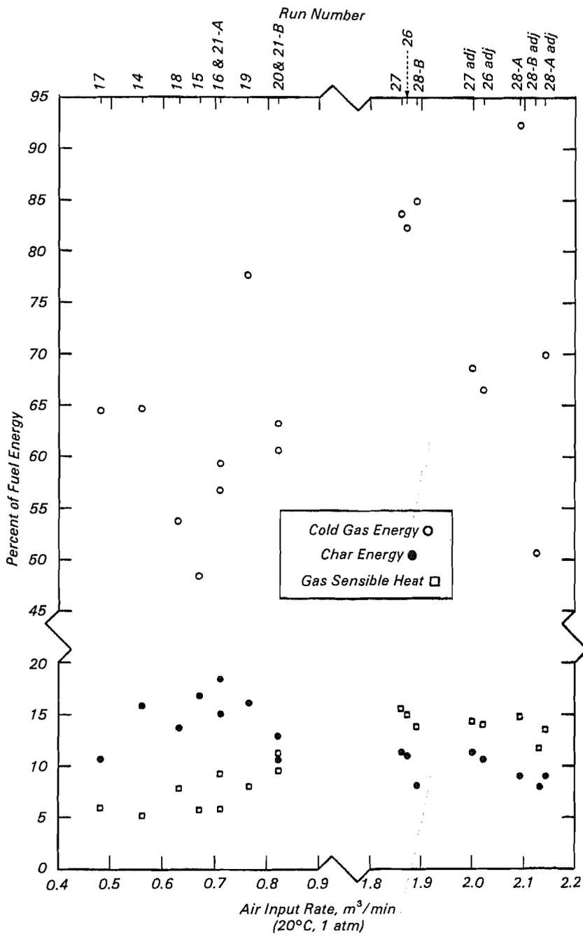
Figure 3. Gasifier efficiencies vs. air input rate.
