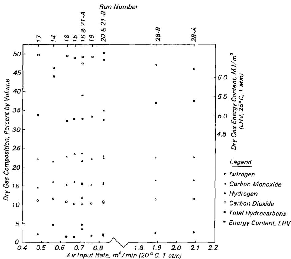
Figure 2. Producer gas composition vs. air input rate.
