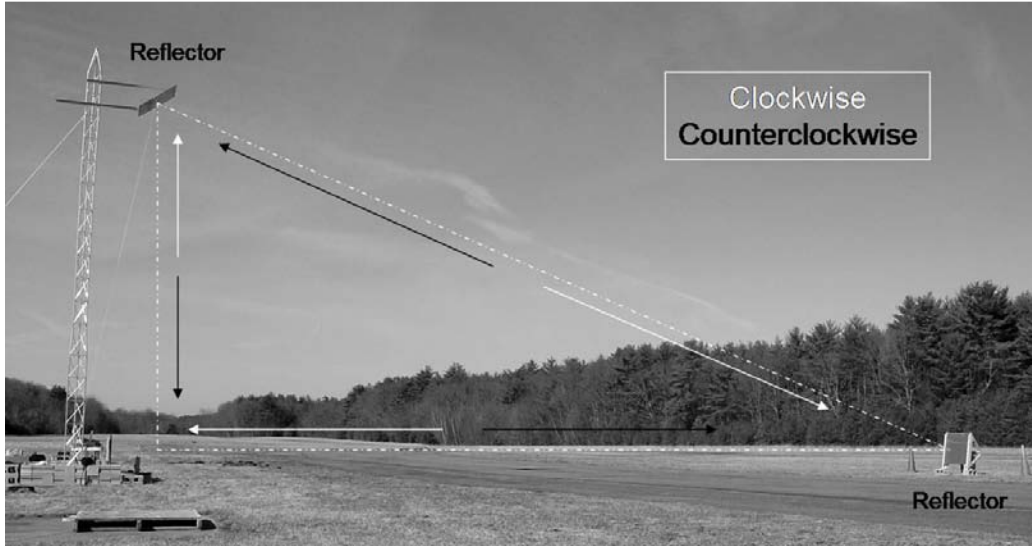
Figure 3. Test Equipment Setup Showing Directions of Signal Transmission
