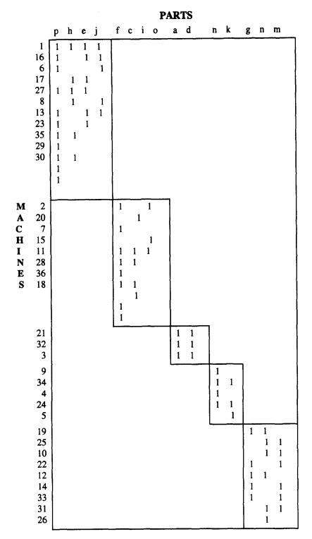
Figure 1. Machine-Part Matrix
