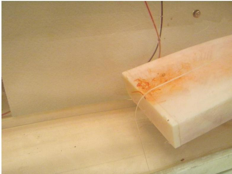
**Figure 19. At the highest  $\alpha$  experimented, it is clear the tabs do nothing to attenuate the vortex sheds.**
