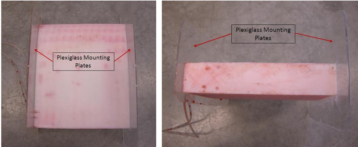
**Figure 4. Here the model is shown attached to mounting plates that gave the body a two-dimensional nature to the flow.**
