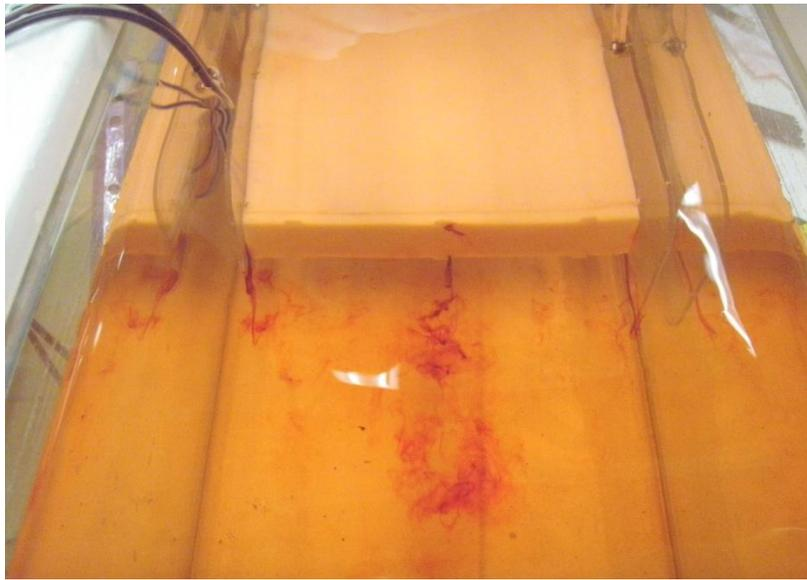
**Figure 17. The tab model managed to output dye from all three spanwise locations and depicts the central wake.**
