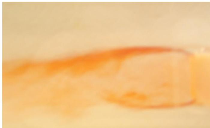
**Figure 11. This vortex was observed directly behind the bluff body with tabs, in perfect comparison to the theoretical model shown in Fig. 10**
