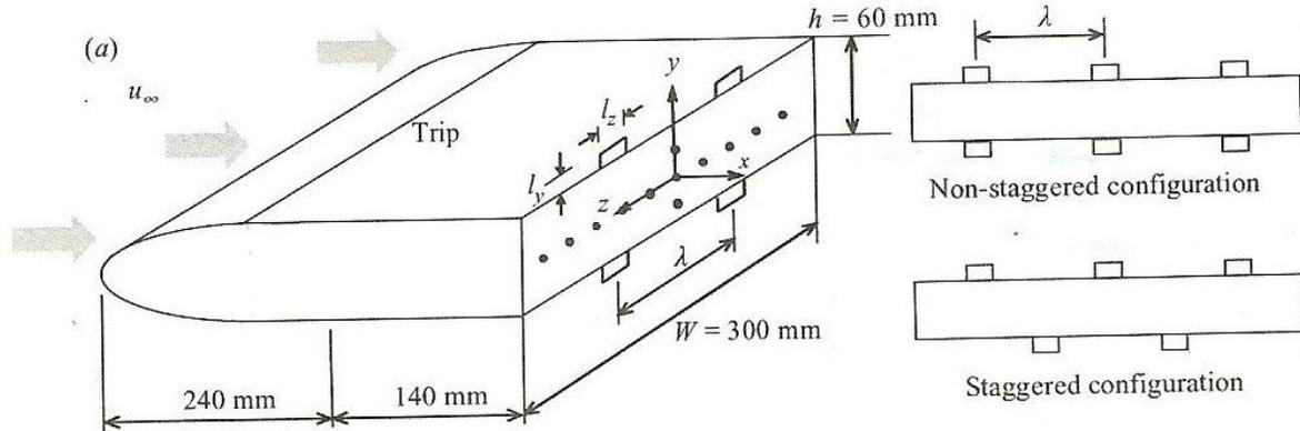
**Figure 1. The model used by Park, et.al is shown here. The model used for the flow visualization study used the same shape with dimensions proportionally modified for a different test section size, and the non-staggered tab configuration.**
