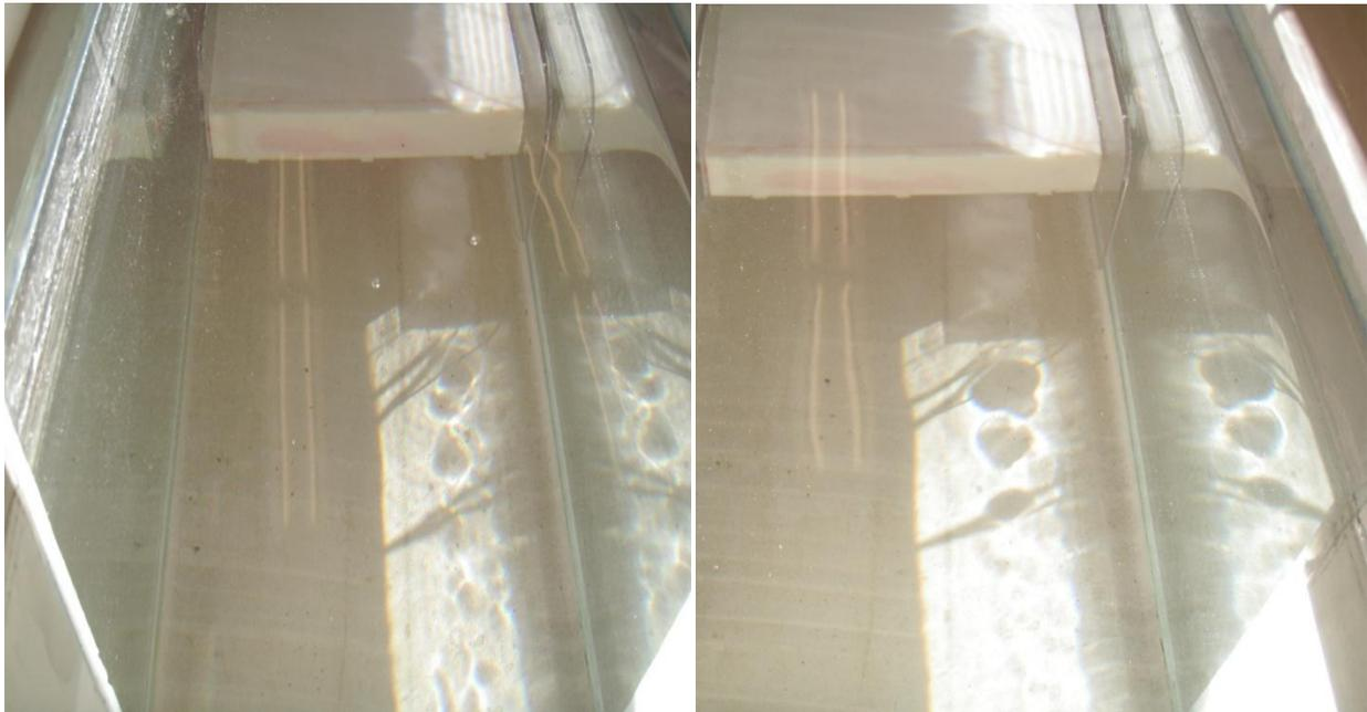
**Figure 14. Views taken from behind and above the model with the tab endplate before introduction of dye to the system uses light and shadows to illuminate the distinct vortex shapes.**
