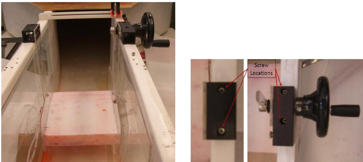
**Figure 7.** The tunnel mounting fixture held the model in place, and connected to the test section via tightened screws.
