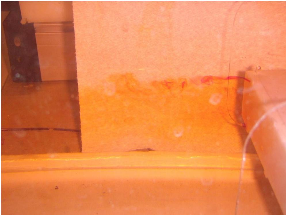
**Figure 16. Karman vortex shedding occurs farther from the trailing edge with the passive control system in place.**
