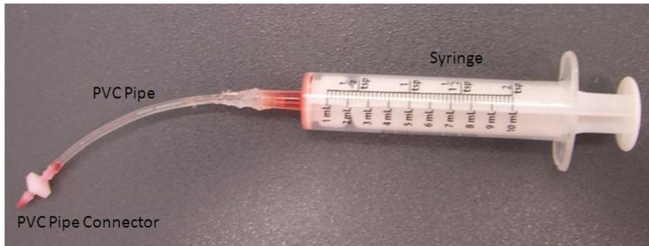
**Figure 3. A syringe filled with dye and connected by PVC tubes to channels in the model provided control of dye flow.**
