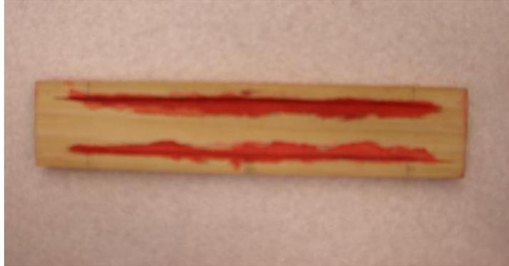
**Figure 6.** This wooden end plate was attached to the blunt trailing edge during the control test.
