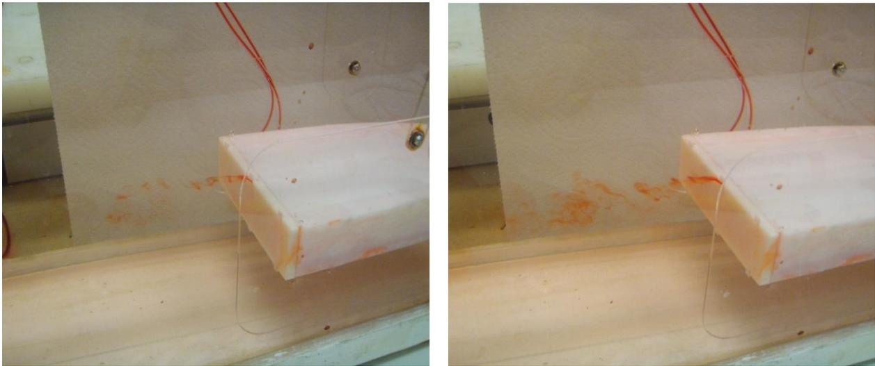
**Figure 12. The Karman vortex sheds developed in distinct, separate groups behind the bluff body fitted with the passive control device.**
