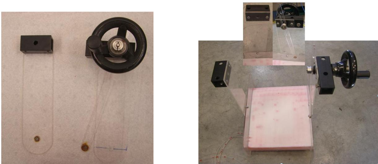
**Figure 5. A fixture of Plexiglass and connecting screws was in use to hold models in the water tunnel.**
