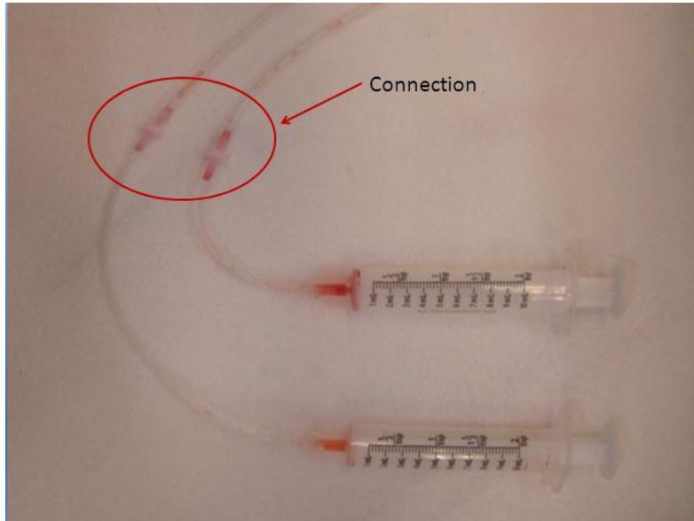
**Figure 8. The model's built-in dye tubes were connected to the pressurization system via PVC tubing.**
