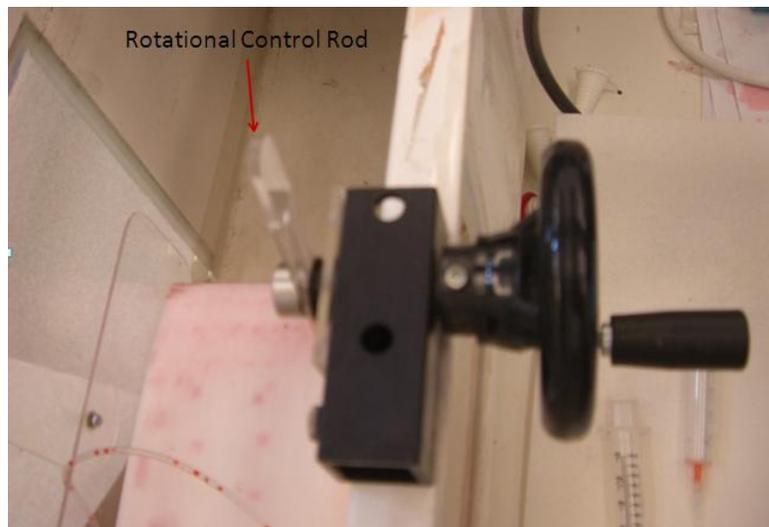
**Figure 9. This rotational control rod controlled the orientation of the model with respect to freestream flow.**
