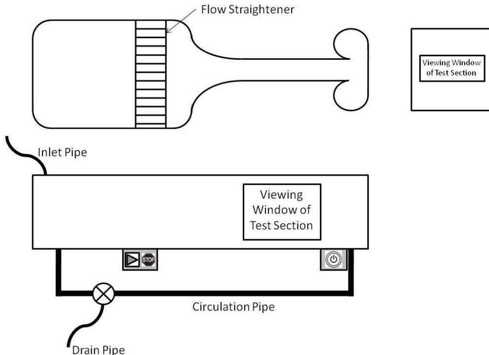
**Figure 2. The top, back, and side views of the water tunnel are shown here.**
