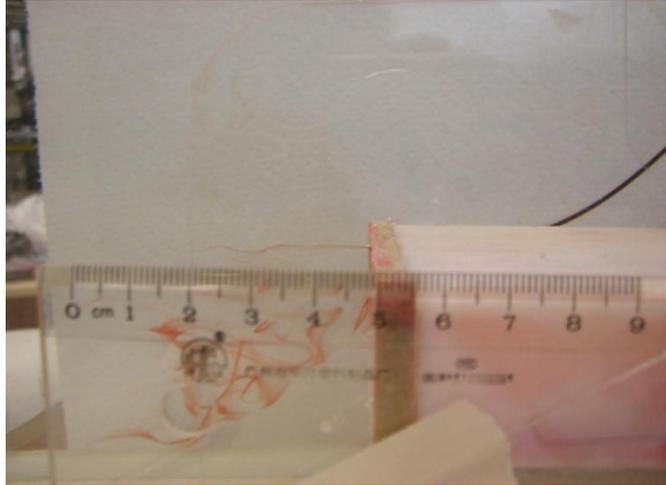
**Figure 13. Vortices behind the bluff body with the control endplate affixed displayed more random, strong, and turbulent vortex formation.**
