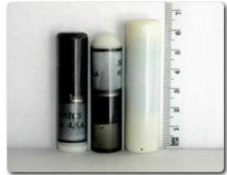
Figure 2: Sonotronics 73 kHz transmitter (middle)
