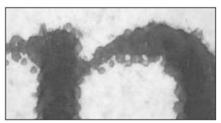
Photo 7 - The serrated edges around the type are a sure sign that this is a gravure printed product.
