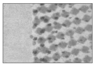
Photo 1 – This offset printed magazine shows relatively consistent halftone images and a smooth gradation in the black.
