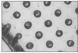
Photo 11 - The doughnut tones, combined with the halo on the type makes one suspect this is a flexo sample.
