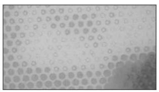
Photo 8 – These tones show the doughnut center typical of gravure printing. This sample used laser engraved cylinders.
