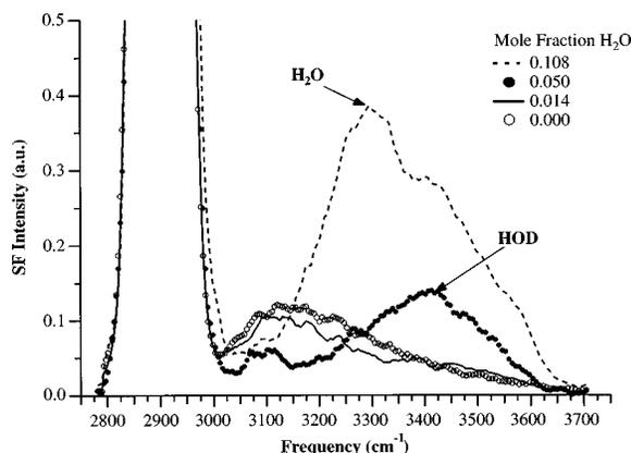
FIG. 2. VSGF spectra from the  $\text{CCl}_4/\text{H}_2\text{O}$  interface with 1.0 mM SDS in the aqueous phase for low mole fractions of  $\text{H}_2\text{O}$  under *S*-sf, *S*-vis, *P*-ir polarization conditions.
