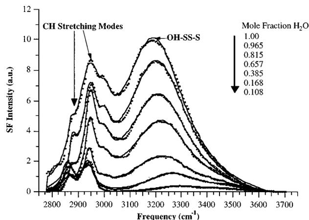
FIG. 1. VSF spectra from the  $\text{CCl}_4/\text{H}_2\text{O}$  interface with 1.0 mM SDS in the aqueous phase as a function of mole fraction of  $\text{H}_2\text{O}$  under *S*-sf, *S*-vis, *P*-ir polarization conditions. Solid lines are a spectral fit to the data.
