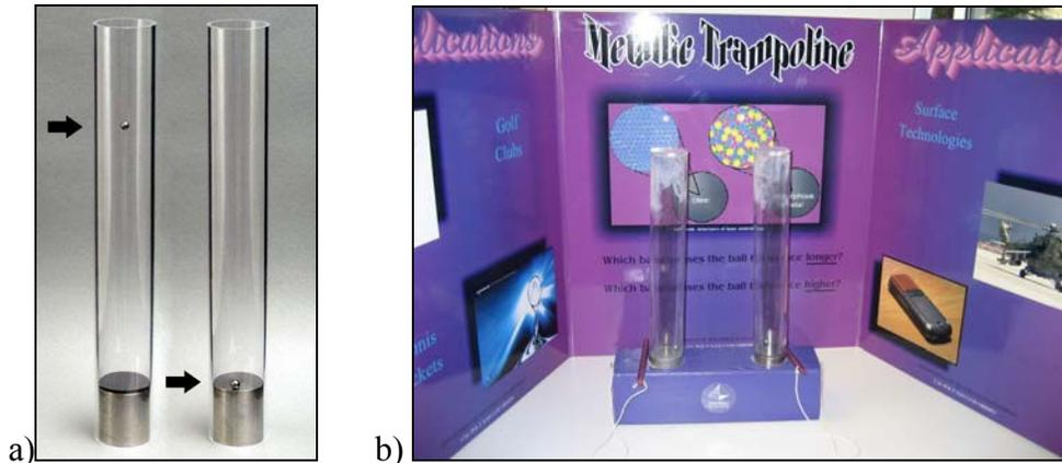
**Figure 5.** a) The Atomic Trampoline demo compares the effect (i.e., coefficient of restitution) of a steel and amorphous metal base when ball bearings are dropped from the top of the plastic tubes. b) The Metallic Trampoline display was designed to be all one piece and uses magnetic wands to transport the ball bearings to the top.
