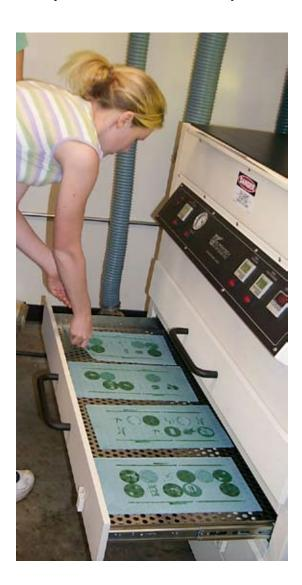
If using one of the mask systems, you must expose the plate through the mask to form the graphics. This is what creates the hard part of the plate—the part that remains after processing.
