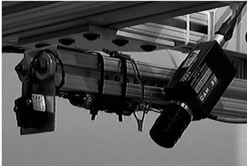
Figure 4: Laser (left) and camera (right) used in PRIME sensor. The laser generates a plane of light using a cylindrical lens. A bandpass optical filter on the camera yields distinct imagery of the laser plane as it intersects objects in the scene.
