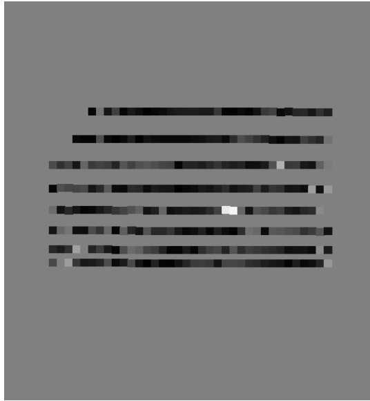
Figure 12: Residual error of a 3rd order (type 4) Z calibration model. Mean = 0.002 in. Gray levels of each block are scaled to span the extremes of the residual errors in this model (maximum = 0.013 in).
