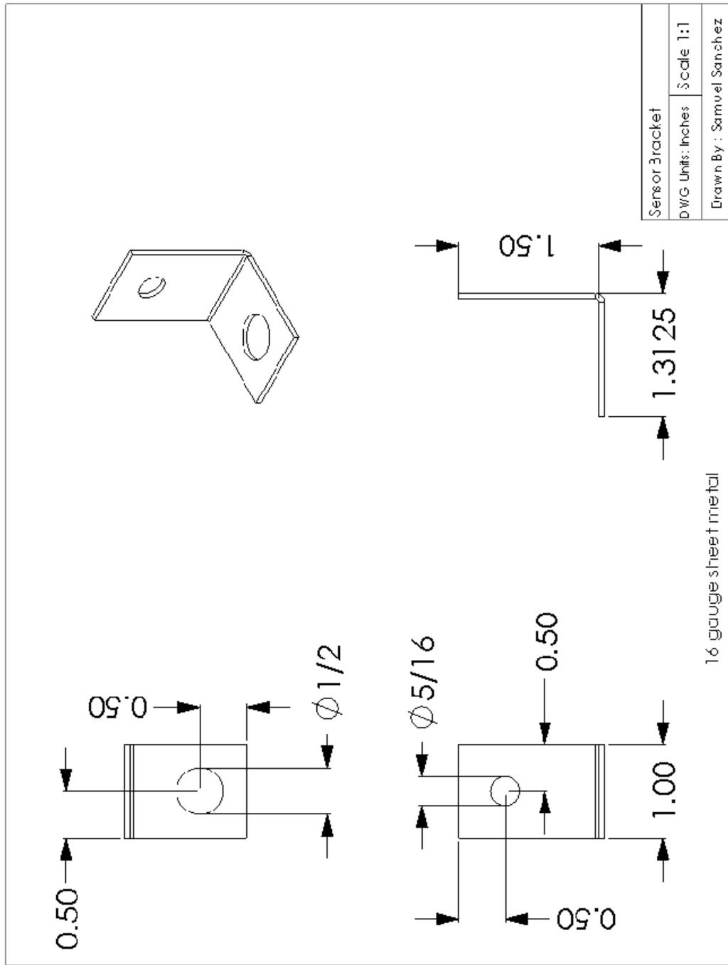
Figure 31: Sensor Bracket
