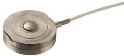
Figure 5: Load cell purchased from Measurement Specialties
