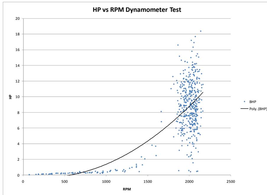
Figure 18: Test 2 of HP vs RPM dynamometer test
