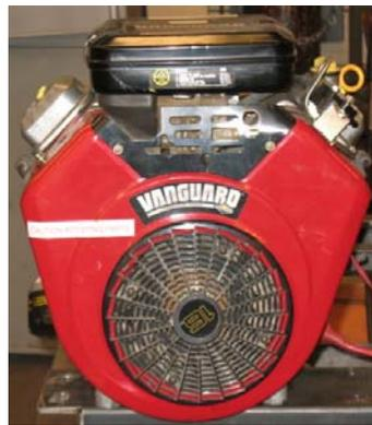
Figure 3: 16Hp Briggs and Stratton Engine
