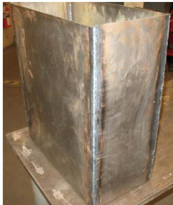
Figure 14: Reservoir with 5 walls welded
