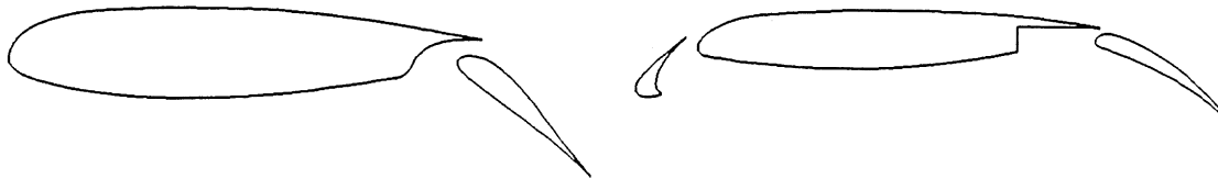
Fig. 2. Lift-enhancing tab geometry in main-element cove on two-element airfoil.
