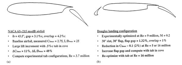
Fig. 3. Multi-element airfoil geometries: (a) baseline two-element airfoil [5]; (b) baseline three-element airfoil [1].
