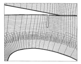
Fig. 6. Close-up of main-element cove showing grid resolution in the vicinity of the tab.
