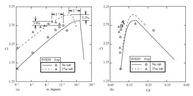
Fig. 9. Lift and drag of two-element airfoil with and without a 1%c tab;  $\delta_f = 43.5^\circ$ ; gap = 3.1%c, overlap = 4.2%c, Re<sub>c</sub> =  $3.7 \times 10^6$ . (a) Lift coefficient versus angle of attack; (b) Lift coefficient versus drag coefficient.
