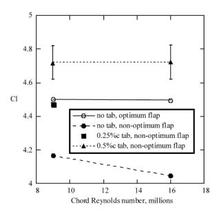
Fig. 14. Effect of tab height on lift for the three-element airfoil,  $\alpha = 25^{\circ}$ ; optimum flap configuration:  $\delta_f = 30.0^{\circ}$ , gap = 1.32%c; non-optimum flap configuration:  $\delta_f = 45.0^{\circ}$ , Gap = 2.18%c.
