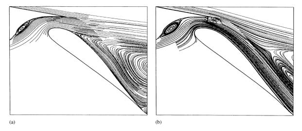
Fig. 8. Computed streamlines near flap for two-element airfoil;  $\delta_f = 43.5^{\circ}$ , gap = 3.1%c, overlap = 4.2%c, Re<sub>c</sub> =  $3.7 \times 10^6$ : (a) baseline airfoil with no tab,  $\alpha = 8.43^{\circ}$ ; (b) airfoil with 1%-c tab located at 1%-c from trailing edge,  $\alpha = 8.5^{\circ}$ .
