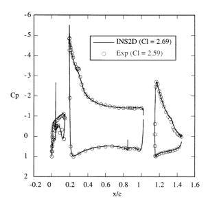
Fig. 12. Computed and measured pressure distributions for baseline three-element airfoil with a tab; optimized flap configuration; gap = 1.32%c,  $\alpha = 4^{\circ}$ ,  $Re_c = 9.0 \times 10^6$ .
