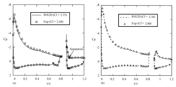
Fig. 7. Computed and measured pressure distributions for two-element airfoil;  $\delta_f = 43.5^\circ$ , gap = 3.1%c, overlap = 4.2%c, Re<sub>c</sub> =  $3.7 \times 10^6$ : (a) baseline airfoil with no tab,  $\alpha = 8.43^\circ$ ; (b) airfoil with 1%-c tab located at 1%-c from trailing edge,  $\alpha = 8.5^\circ$ .
