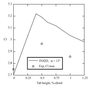
Fig. 10. Effect of tab height on lift; tab at main-element trailing edge on two-element airfoil;  $\delta_f = 43.5^{\circ}$ , gap = 3.1%c, overlap = 4.2%c, Re<sub>c</sub> =  $3.7 \times 10^6$ .
