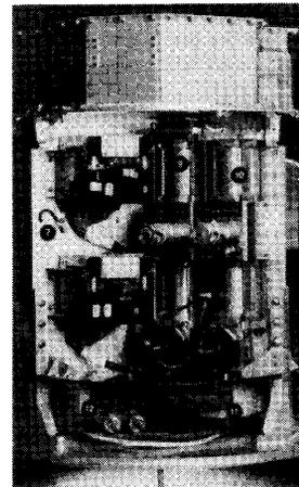
Seen in this second view are the: (7) temperature sensor for EDAS (other sensors located in the GASCAN feed information about pressure, sound and light to EDAS), (8) data recorders for the fluid behavior experiment, (9) fluid behavior experiment: wetting fluid cylinder, (10) fluid behavior experiment: nonwetting cylinder, (11) power distribution control hardware, (12) temperature controller for the zeolite crystal growth experiment.
