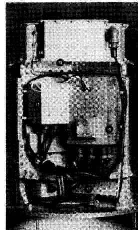
In this third view are seen the: (13) power converter for the fluid behavior experiment, (14) over-pressure vent lines for the battery compartment, (15) film fogging experiment (other film holders are located in other spots and in other orientations in the GASCAN), (16) controller for the fluid behavior experiment, (17) triaxial precision accelerometer. The GASCAN structure seen here will be delivered to NASA shortly before launch to be inserted into an external aluminum canister.
